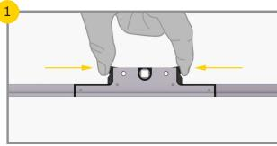
Grip the gearbox with other hand locating thumb on the square drive gear area of the gearbox cassette.
