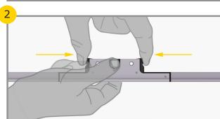
Whist holding in the gearbox cassette clips, pull up on the cassette using the thumb of the other hand to aid disengagement.
