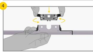
Re-insert cassette ensuring clips re-engage and lock operates correctly.
