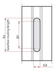
Backset 20 or 22 mm, with cam 8 and 9,5 mm.
