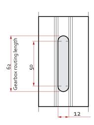
Backset 20 or 22 mm, with cam 8 and 9,5 mm.
