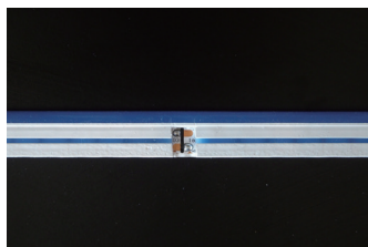
2. Clean and prepare the soldering pads
