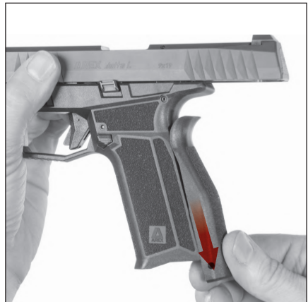
Figure 9 — Removing/installing the backstrap
