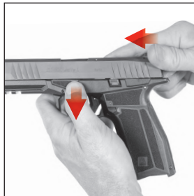
Figure 24 Pulling down the locking latch on both sides of the frame then pushing slide forward
