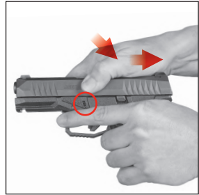
Figure 43 Push the slide down and pull it back seeing the disassembly latch spring up
