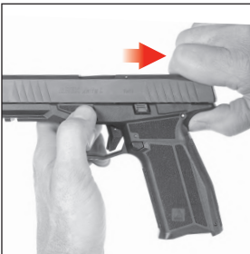
Figure 23 Pulling slide back slightly and holding it
