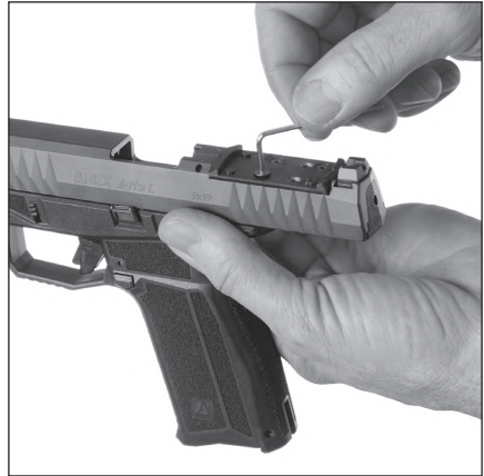
Figure OR6 - Mounting the appropriate interface plate
