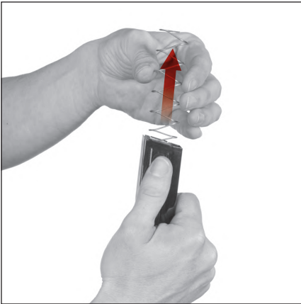
Figure 30 — Removing the spring with follower
