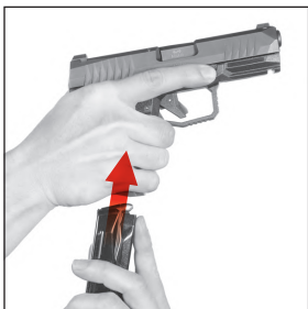
Figure 13 Inserting the magazine
