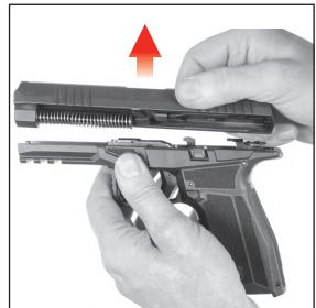
Figure 25 Lifting the slide from the frame
