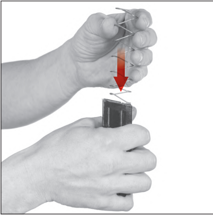
Figure 44 — Insert the follower and spring
