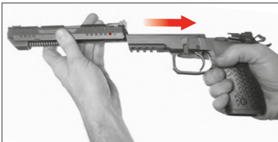
Figure 35 — Mounting the slide on the frame (frame guides aligned with slide grooves)
