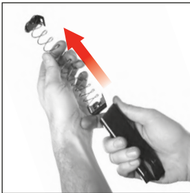
Figure 30 Removing the locking plate with spring and follower
