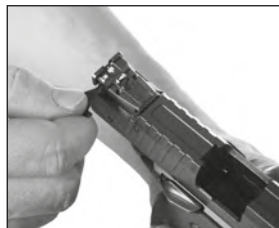
Figure 17 Adjusting the rear sight for windage
