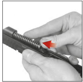
Figure 34 — Compressing the recoil spring, positioning the recoil spring guide in front of barrel's guiding lug
