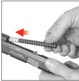
Figure 33 — Inserting the exposed end of the recoil spring into the front of the slide
