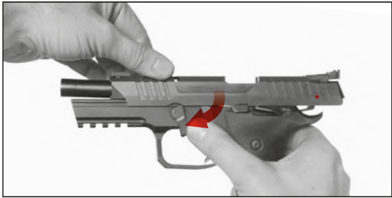
Figure 23 — locking the slide Figure 24 — Rotating the disassembly lever downwards
