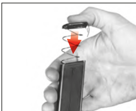
Figure 37-Insert the spring with follower and locking plate attached to it
