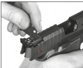
Figure 16 Adjusting the rear sight for elevation
