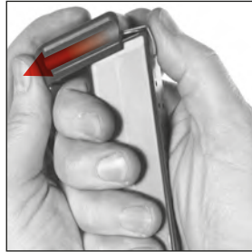
Figure 29 Sliding the floorplate forward Caution: spring under tension!
