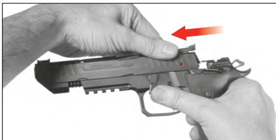
Figure 25 — Removing the slide from the frame by sliding it forward
