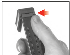
Figure 39-Check the floorplate is arrested by the locking plate
