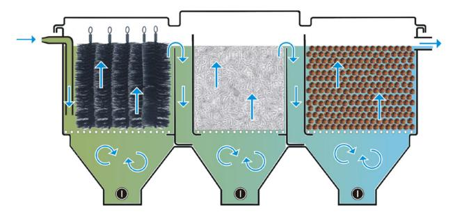
Model BIOklar Move 15 has 3 filtering chambers:
