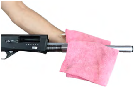
◀ Push the latch (cartridge drop lever) under the trigger group. Pull back the bolt handle. Clean the outer surface of magazine tube with a soft cloth.
