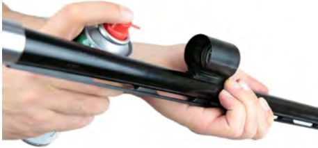
◀ Clean the gas port by using a gun cleaning oil and soft cloth.
