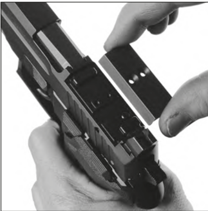
Figure T6 - Removing the Arex Optics Ready cover plate
