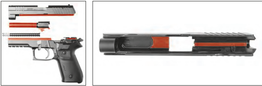
Figure 34 — Medium lubrication points marked red (view of the slide underside)
