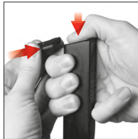
Figure 33 Hold the locking plate in the magazine body while sliding the floorplate onto guides until detent clicks in place
