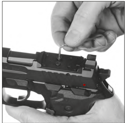
Figure T7 - Mounting the appropriate interface plate
