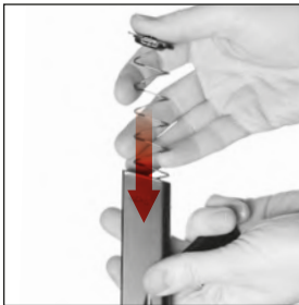
Figure 32 Insert the follower, spring, and locking plate
