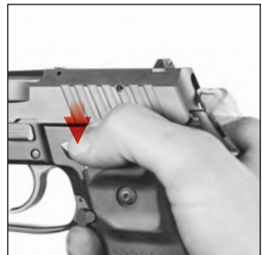
Figure 12 Decocking the hammer
