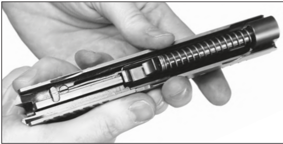
Figure 29 — Reassembling the recoil spring onto the barrel and slide (wide end of the spring guide located in front of barrel's guiding lug)
