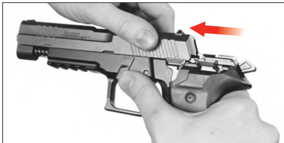
Figure 22 — Removing the slide from the frame by sliding it forward
