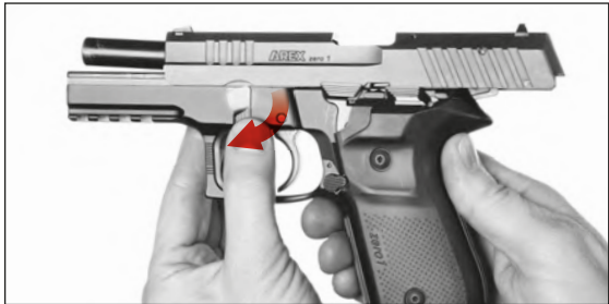
Figure 21 — Rotating the disassembly lever
