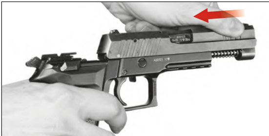
Figure 30 — Mounting the slide on the frame (frame guides aligned with slide grooves)
