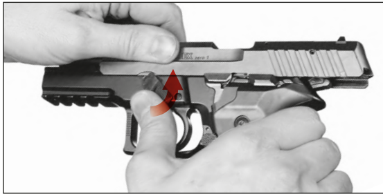
Figure 31 — Pivot the disassembly lever counter clockwise
